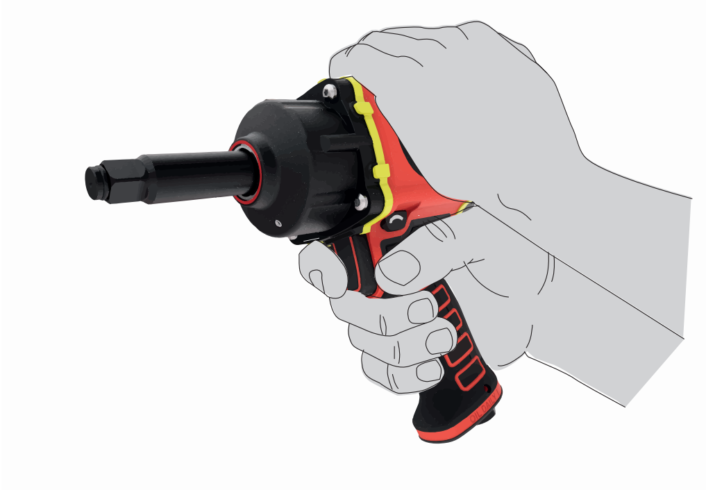
figure 5 : Correct position to handle the tool
